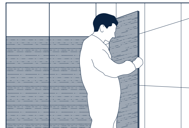
13 | Laying of a protective cardboard on the installed wall
